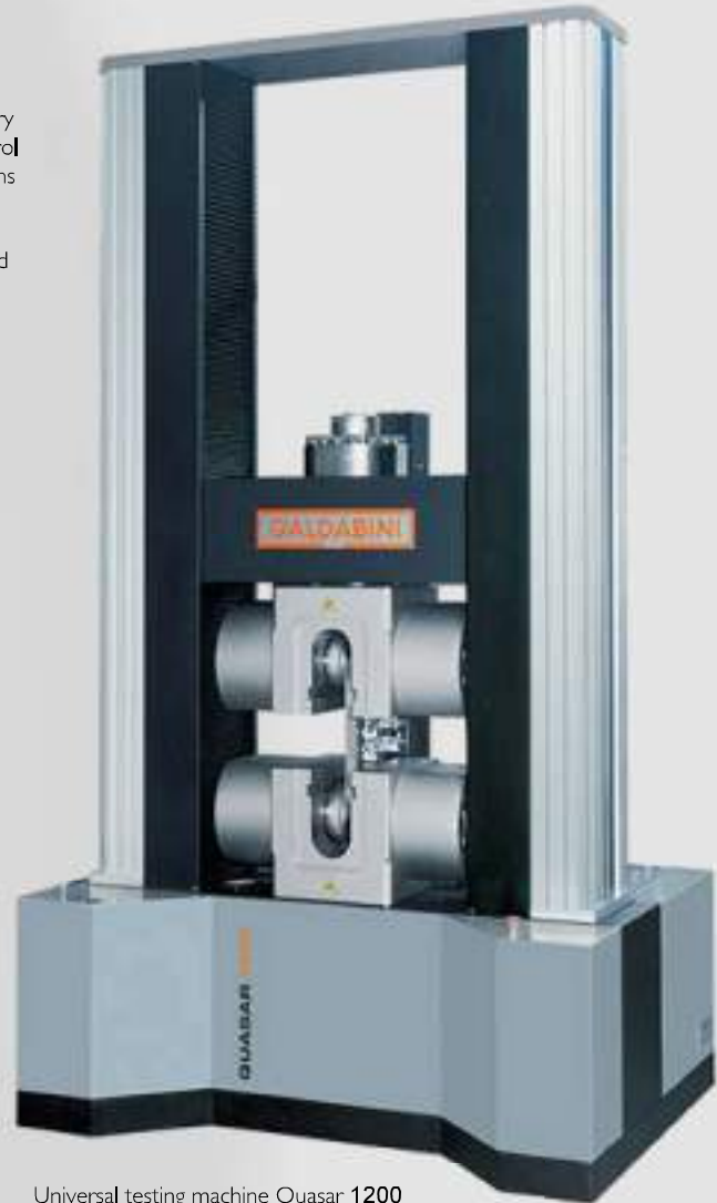
Universal testing machine Quasar 1200 with Hydraulic parallel closing grip and "Micron" extensometer
